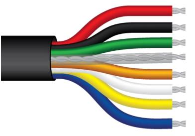
Red: High side of differential channel (positive lead for Opsensor)
