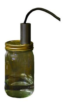
Apogee oxygen sensor mounted in a sealed chamber over water. For measurements in environments where relative humidity is 100 %, sensors should be calibrated in conditions where relative humidity is 100 % in order to account for any humidity effects on sensor electronics.
